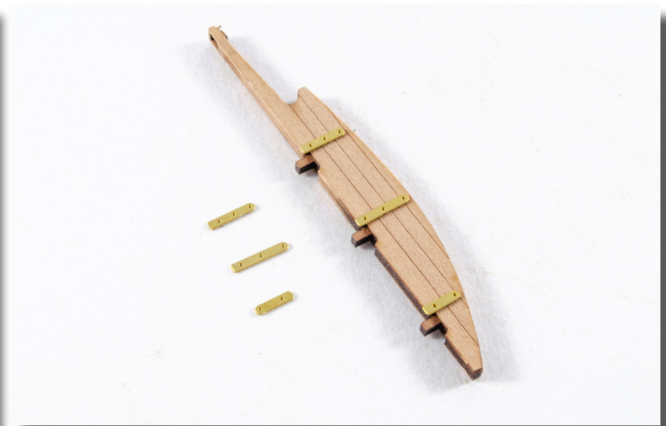
123. Remove parts #PE-24, #PE-25 and #PE-26 from the PE sheet, and glue into their respective positions on the rudder, using CA.
