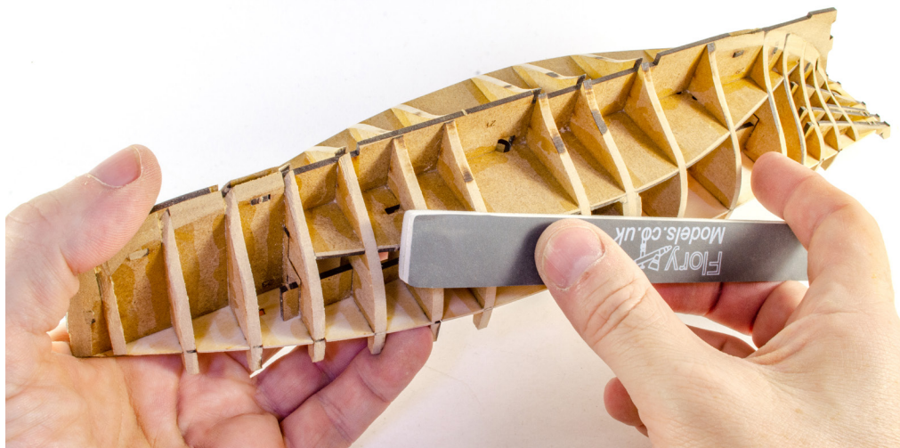
48. Before the hull can be planked, it needs to be sanded smooth so a plank will lie along it with maximum contact to all areas. This process is called 'fairing'. Use sandpaper or a flexible sanding stick to smooth off the hull to achieve this. IMPORTANT: As with any timber sanding, we recommend a face mark. MDF dust isn't very pleasant, so protect yourself!
