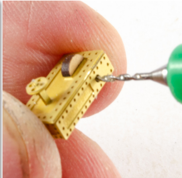
180. Use a 1mm drill bit to drill through the hole in the side of the assembly, and into the MDF.
