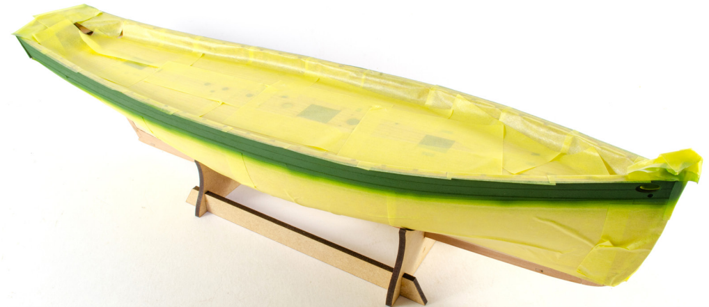
112. On our Erycina prototype, we decided to paint the upper outer bulwarks in green. You can use whatever colour you choose. First of all, the bulwark area was brushed with a thin coat of polyurethane varnish and allowed to dry. As we airbrushed Tamiya XF-5 Flat Green, we first masked the model so that only the upper bulwark was visible. Green was then airbrushed in thin coats until a nice, solid coat was achieved.
