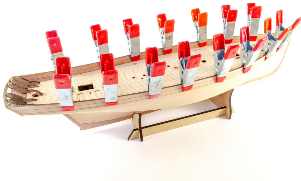
97. Use small clamps to hold the deck down around the edges until properly dry.
