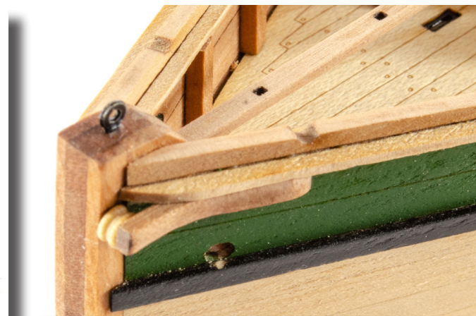
209. Glue parts #93 into place as shown, on the engraved marks on the gunwale. Also note that the Bow Roller has been fitted. Glue #47 into position using plan as reference. Now use the short length of 1mm brass wire which is long enough to fit through hole in prow and rest up against the part you just fitted. The brass wire needs to be flush with other side of prow. Fit the wire, trapping the 2.5mm thimble between the prow and the knee.
