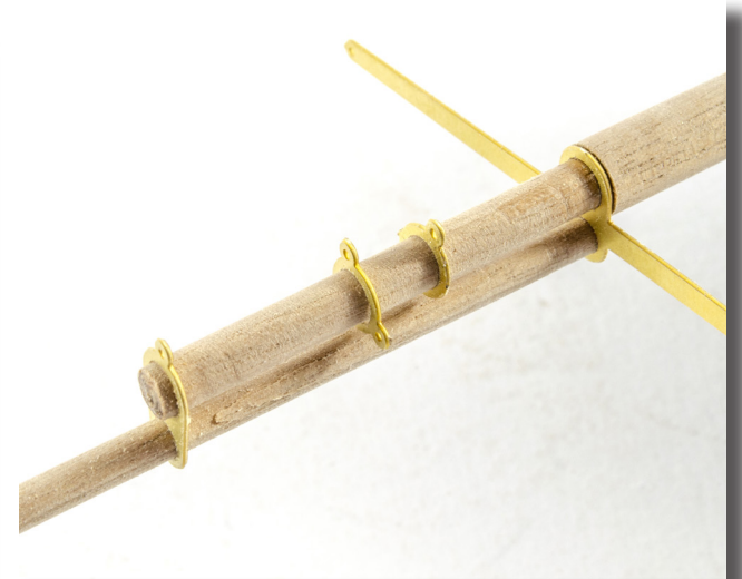
217. Fit the upper and lower sections together, first trapping the PE parts as can be seen here.
