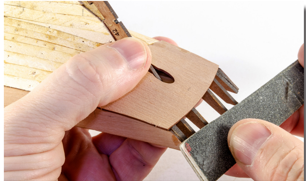
67. Remove part 76 from the 1mm wood sheet. This is called the stern board. The engraved side will face inwards.
