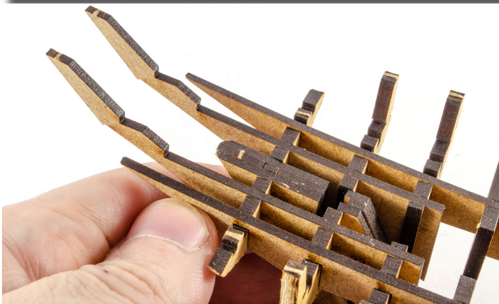
35. These now dry fit (no glue) into the innermost slots at the back (stern) of the boat, as shown here, through the slots in bulkheads 14, 15, and 16.
