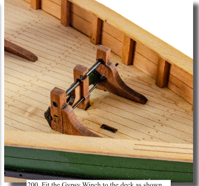
200. Fit the Gypsy Winch to the deck as shown.
