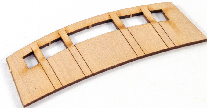
68. Using sandpaper or a flexible sanding stick, sand the stern timbers as shown so they curve from left to right. Not much sanding is required here.
