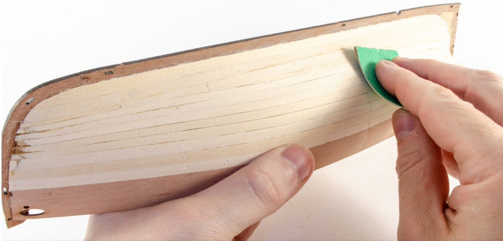
70. Use a suitable grade sandpaper, such as 110 grit, and sand the hull smooth, removing any edges between the planks, and the plank to bulwark transition etc. Run your fingers along the hull to check for any unevenness, as this can be as good an indicator than simply just visually checking.
