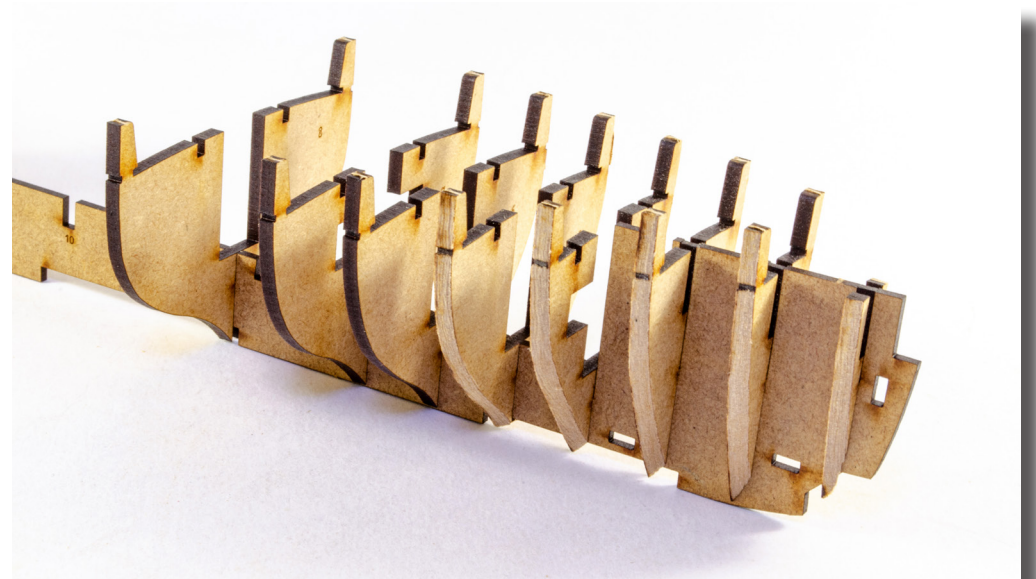
12. Dry fit (no glue) bulkheads 1 through to 8 into the correct keel slots. The first 5 bevelled bulkheads must have the bevel pointing towards the front (bow) of the boat, as clearly seen here.
