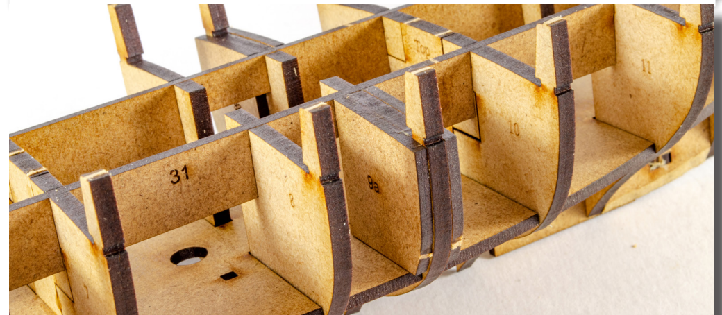
33. Glue these into place on either side of bulkhead #9, so they sit on the lower deck and against parts 31 that you just fitted.
