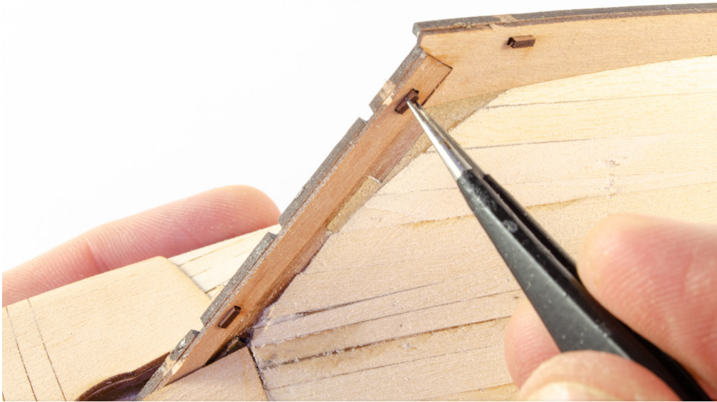
82. Glue the pegs into place and fit the remaining part #66 to the opposite side of the keel.
