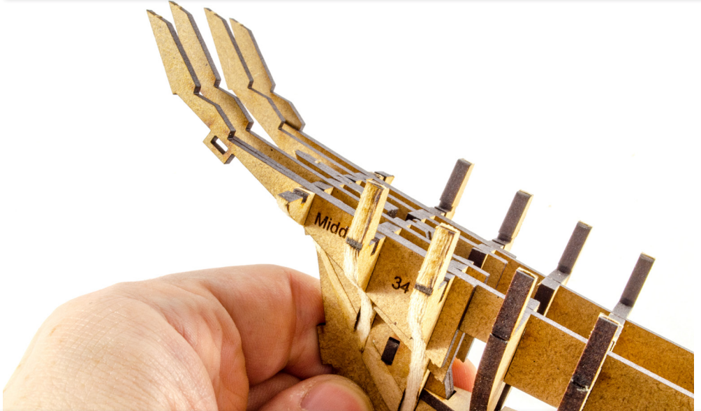
37. Slot these into the same bulkheads as the previous parts, in the next slots along.
