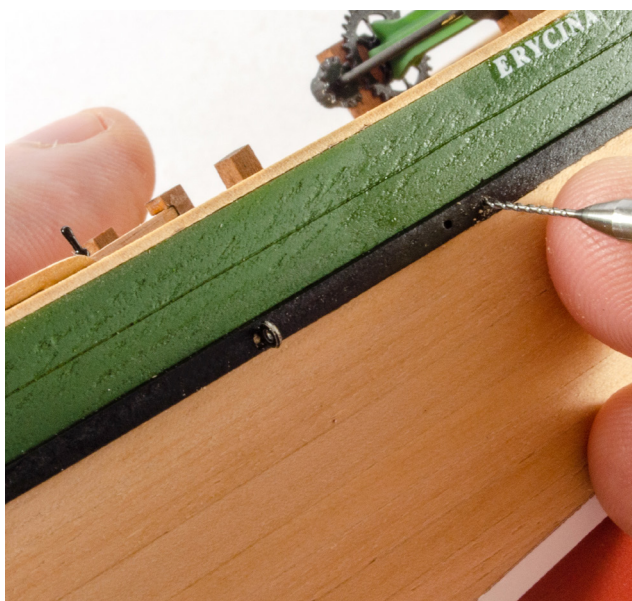
211. Using a 0.8mm drill bit, drill through the holes in the lower rail, but at about 45 degrees, so the drill will come out above the level of the deck.
