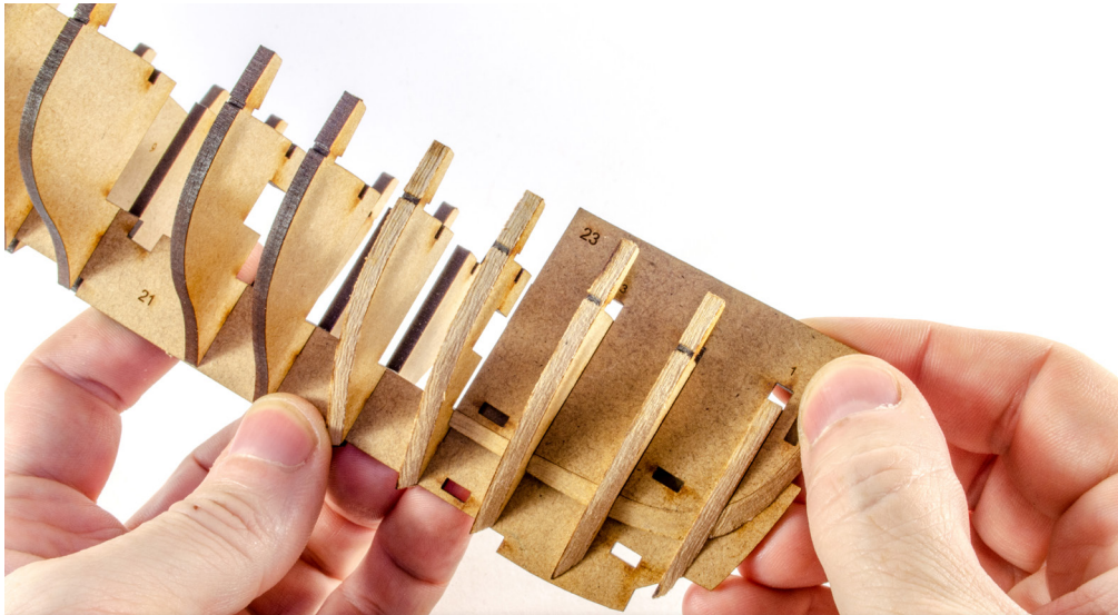
17. You can now glue those parts into position at the front (bow) of the boat, as seen here. Glue to the keel and not to the bulkheads. Of course, the bevelled edges face outwards.
