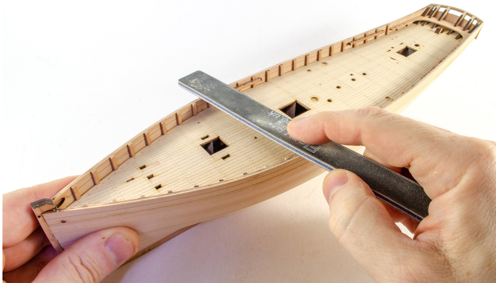
109. Use a rigid sanding stick or some sandpaper wrapped around a steel rule and draw this along the tops of the bulwarks to flatten the tops and make them even. This shouldn't take much work to achieve.
