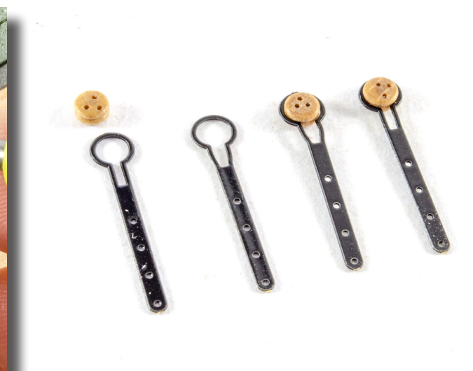
212. From the PE sheet, remove parts #PE-19 and #PE-20. You will also need your 3mm deadeyes. Assembling these is very easy as these stages show. First, splay the PE slightly so the ring opens up. Now clip the deadeye into position. Now use pliers or tweezers to close up the PE and put back to its original shape.
