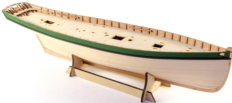
114. For Erycina, we chose black as a contrasting colour which looks good for a working vessel. The rails are then glued into place, so they sit outside the lowermost engraved line which runs along the bottom of the bulwark. NOTE: You will need to bevel the inside front part of each rail so they sit flush to the stem.
