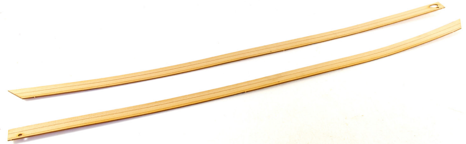
84. From the 0.8mm wood sheet, remove part #102 and #103. These are the outer bulwarks which will form the visible second layer of Erycina.
