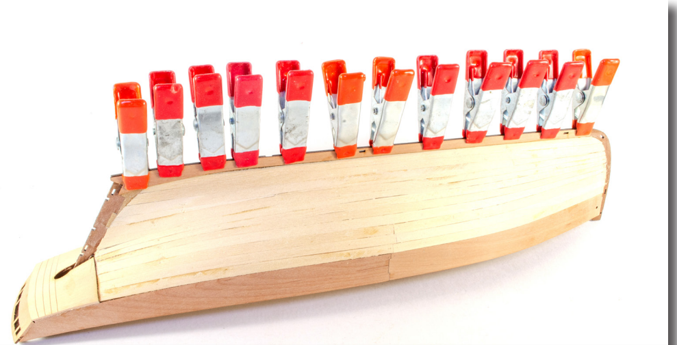
75. Part #65 is the keel rabbet pattern. This glues into position as shown here, so the slots in this and the keel will align. When fitted, this part creates a small rebate for the second layer of planks.
