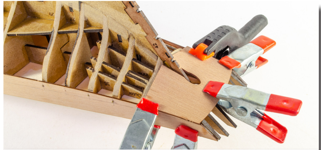
59. On the prototype, we found that soaking the part for 30 mins in hot water, and then clamping in place until dry, really helped with fitting. If you soak this part, you must leave it to dry for at least 12hrs for it to regain its original shape. Pear wood does expand quite a lot when it gets wet. Once dry, glue and pin in place.
