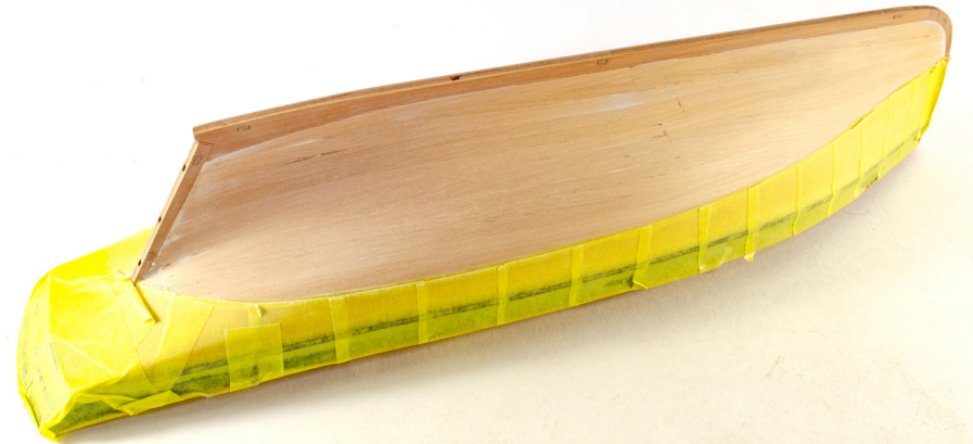
120. Mask all areas above the waterline and then use dilute acrylic wood filler or similar, to fill any imperfections. Sand the area smooth again and repeat until you are happy with the finish.
