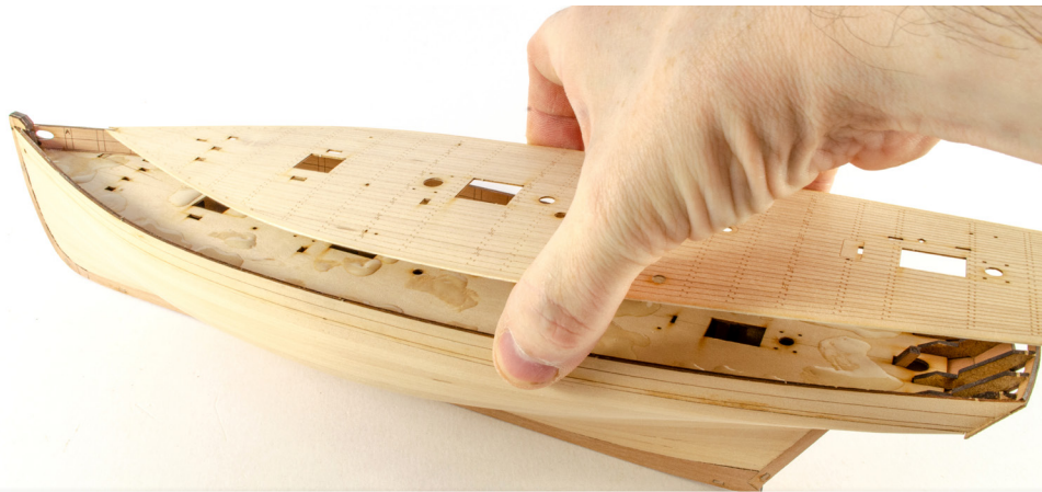
96. Repeatedly test fit the deck onto your model until you are happy that it lies perfectly flat over the contours, and up against the bulwarks. You may need to sand a little from the edges of the deck. On the prototype, I only had to remove the char at the edges for it to fit perfectly. When you are happy with it, glue into position by slotting the bow end into the stem first.
