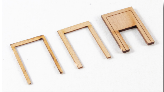
143. COMPANIONWAY: From the 1mm wood sheet, remove part #98. From the 0.6mm wood sheet, remove parts #113 and #114.
